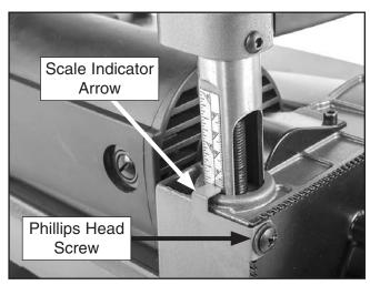
**Figure 35.** Elevation scale components used to calibrate thickness reading.
